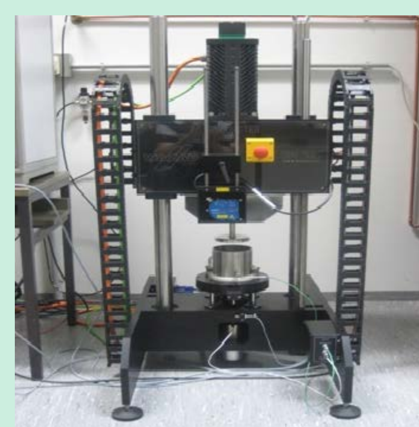
The wear particles are generated by a Wazau TRM 1000 tribometer.
